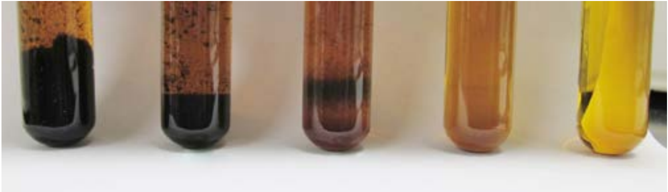
Fig.8—Deposition Tendency Test results – no visible deposits should form
