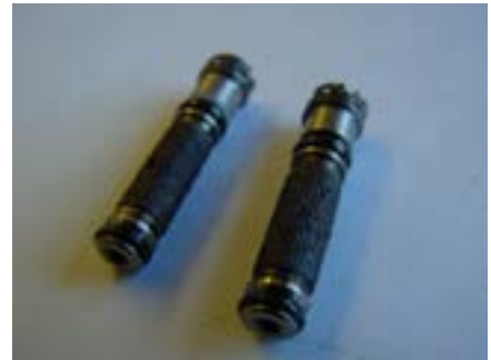
Fig.6—Servo valve strainer plugged with filter fibers from pump discharge filters
